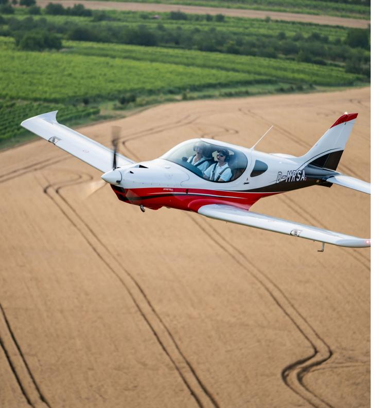
The Bristell RG version has a retractable undercarriage which makes it an ideal airplane for more advanced training and economical cross-country flights. Thanks to the combination of good ergonomic design and the largest cockpit in its category, this airplane is also an ideal option for long cross-country flights. In standard configuration, the BRISTELL RG is equipped with heavy-duty wing spars, making cross-country flights much safer in extreme weather conditions.
