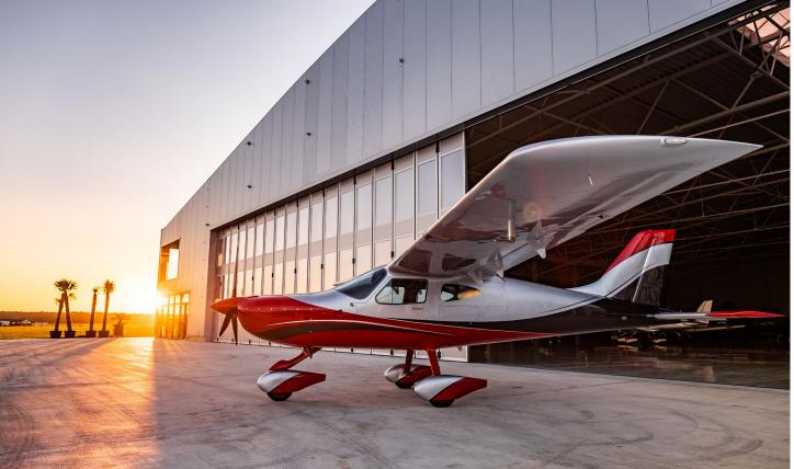
Bristell B8 is an all-metal high-wing without struts and with a steerable nose wheel. The cockpit is 125cm wide. The doors of the cockpit as well as the luggage compartment door are made from composite material.
